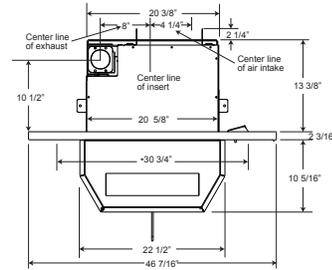
\*In order to install flashing flush to a finished wall and centered within the opening the front opening of the fireplace or enclosure must be this wide.
