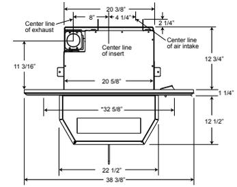
\*In order to install flashing flush to a finished wall and centered within the opening the front opening of the fireplace or enclosure must be this wide.
