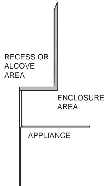
**NOTE:** Recesses or alcoves above the appliance can be made as deep as desired provided the minimum clearances to combustibles are maintained.
