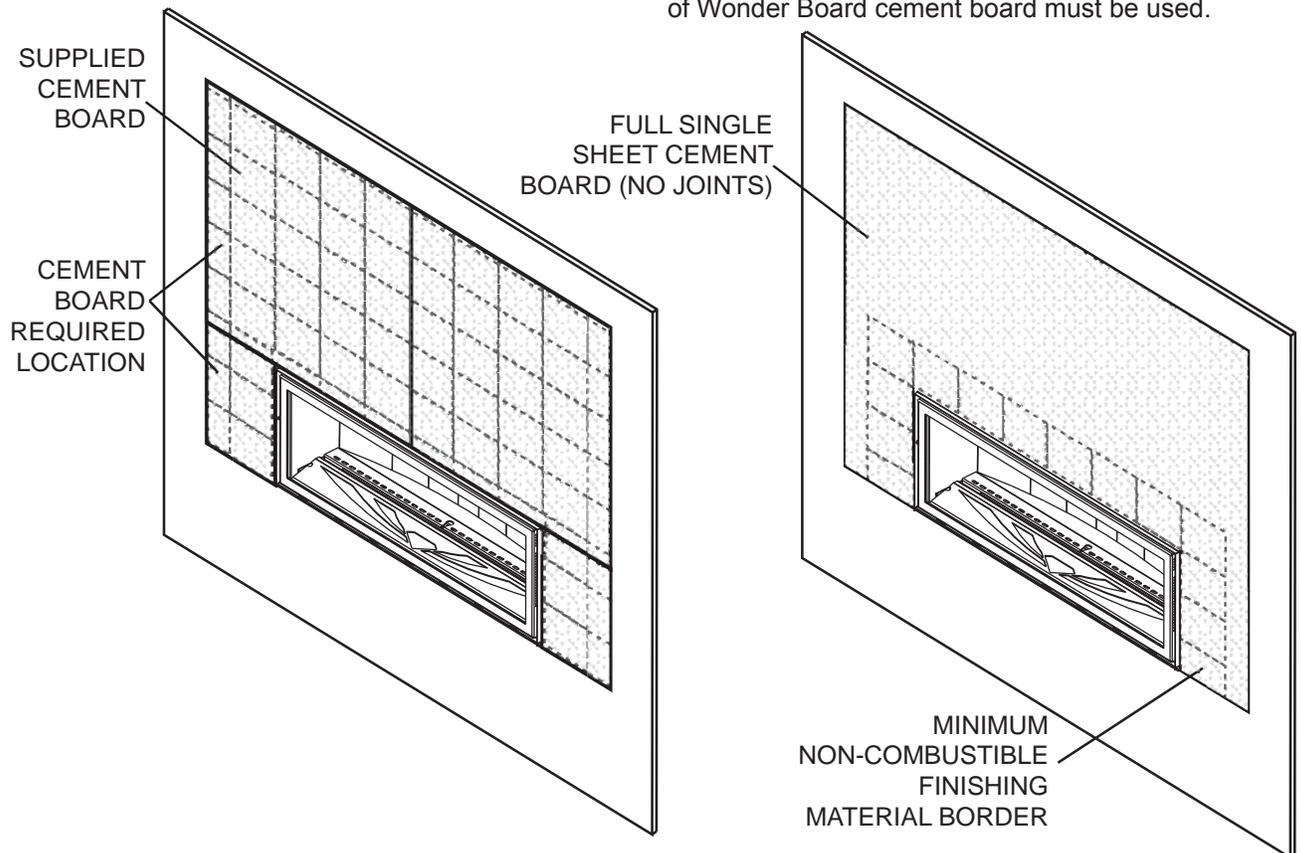
**NOTE:** Keep the securing screws for the cement board a minimum of 6" from the side and top of the door opening. This will allow for any slight movement in the normal operation of the appliance.
