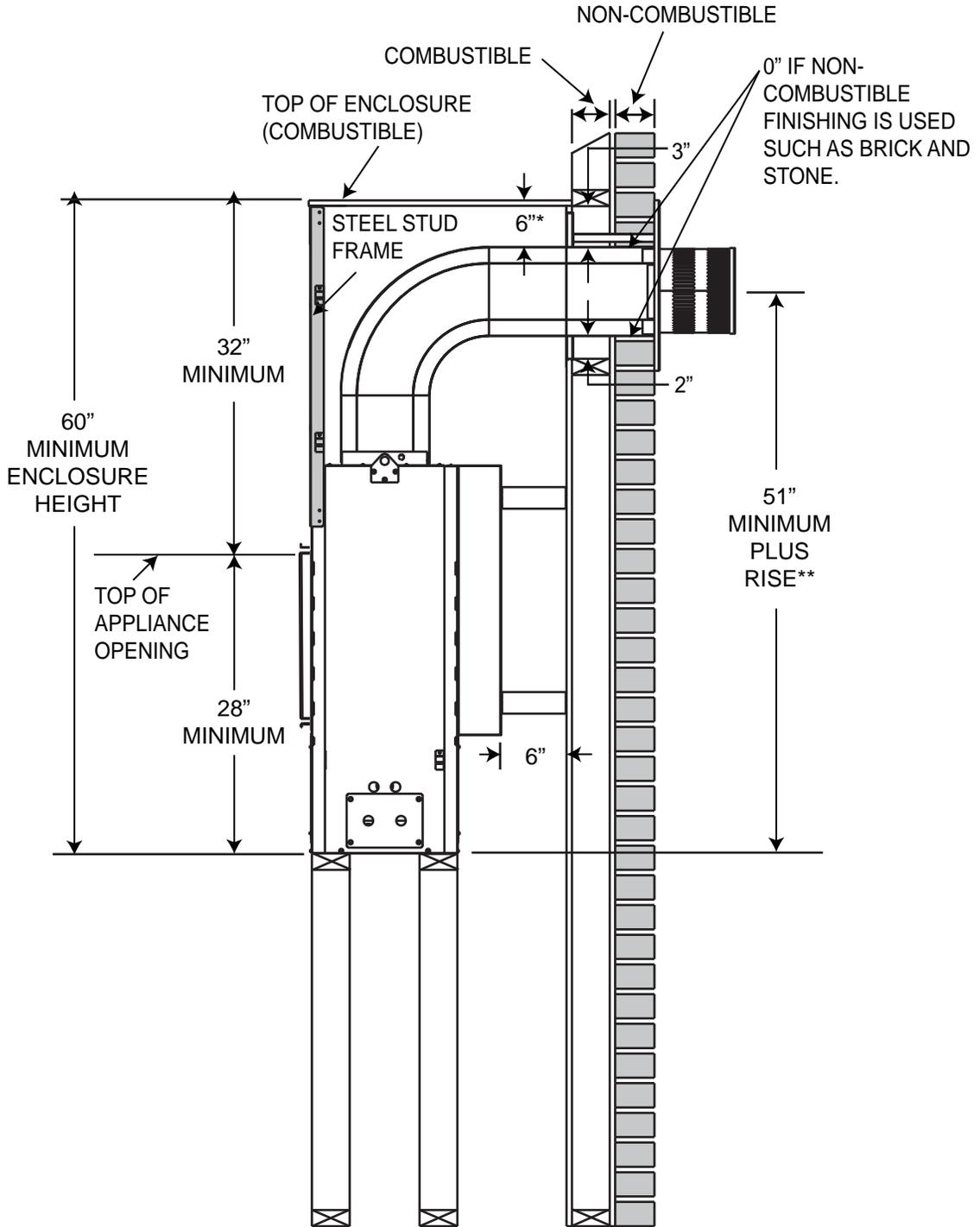
\* Within the appliance enclosure a 6" clearance between the top of the vent pipe and combustible materials is required. All other clearances within the enclosure, including where the vent pipe exits the enclosure are subject to 2" to the sides and bottom and 3" to the top for horizontal and 1" for vertical.
