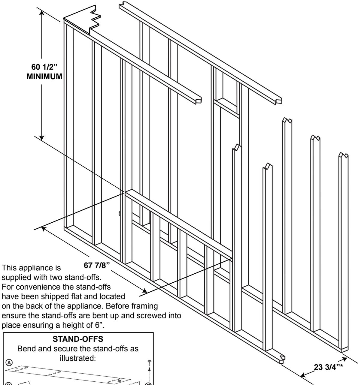
This appliance is supplied with two stand-offs. For convenience the stand-offs have been shipped flat and located on the back of the appliance. Before framing ensure the stand-offs are bent up and screwed into place ensuring a height of 6".
