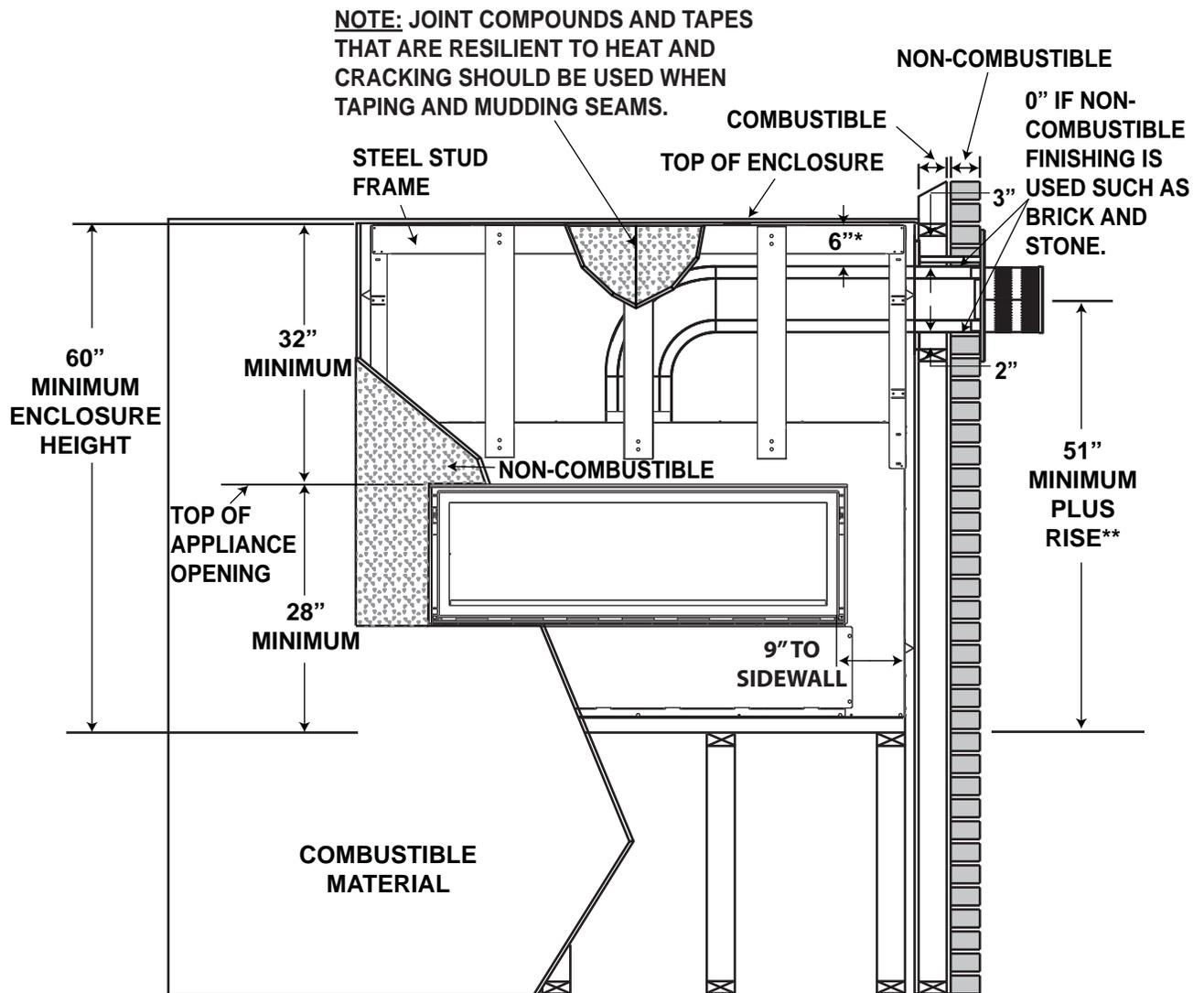
\* Within the appliance enclosure a 6" clearance between the top of the vent pipe and combustible materials is required. All other clearances within the enclosure, including where the vent pipe exits the enclosure are subject to 2" to the sides and bottom and 3" to the top for horizontal and 1" for vertical.
