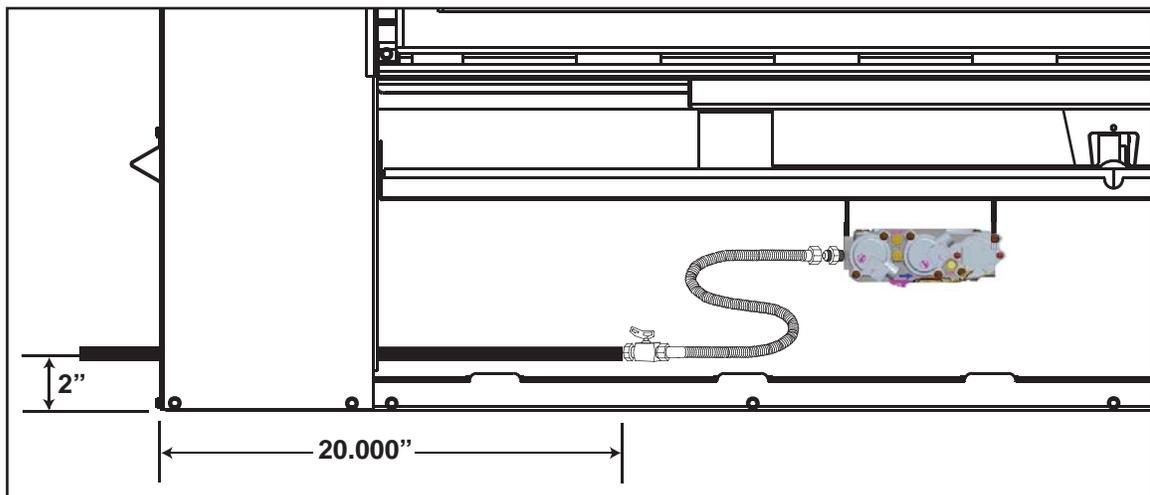
**NOTE:** Connect the gas supply to the 1/2" shut off and flex connector (supplied). Ensure gas supply is secured.
