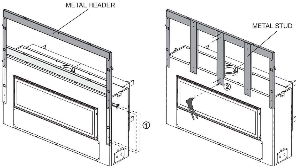
\* When constructing the enclosure allow for finishing material thickness to maintain clearances.
