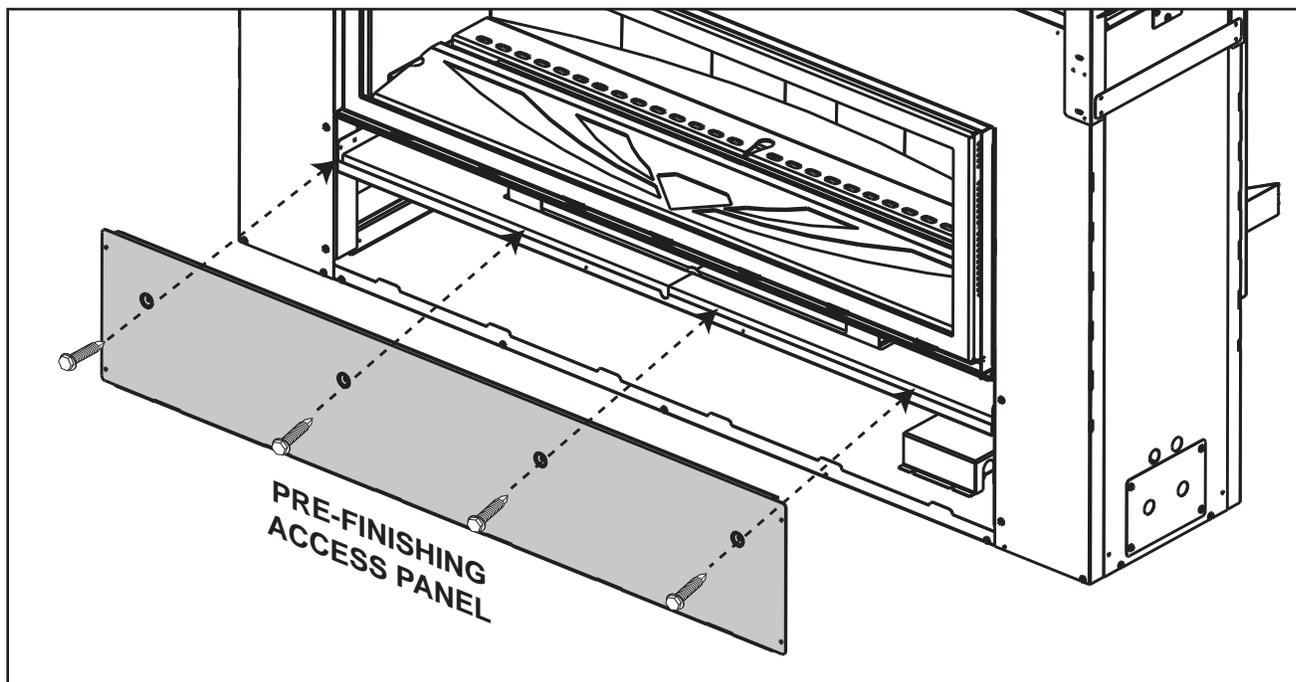
Before finishing in the appliance test the operation using the remote control, cycling it through all of its different modes, see "OPERATION" section. Once finished in, access to the control components can only be done through the inside of the appliance.
