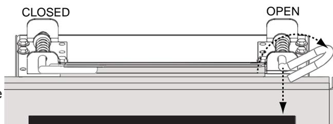
Reverse these steps to re-install the screen and door. Ensure safety screen is installed correctly.
