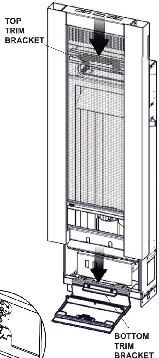
The TORCH® frame has been designed to accommodate finished material thicknesses of 1/2" - 3/4" (13mm - 19mm). If it is necessary to pull the TORCH® frame out to the max. 3/4" (19mm) the magnetic catch will need to be adjusted. Minor adjustment can be made by removing shims from behind the magnet. Major adjustments can be made by moving the magnet to the outside of the panel.
