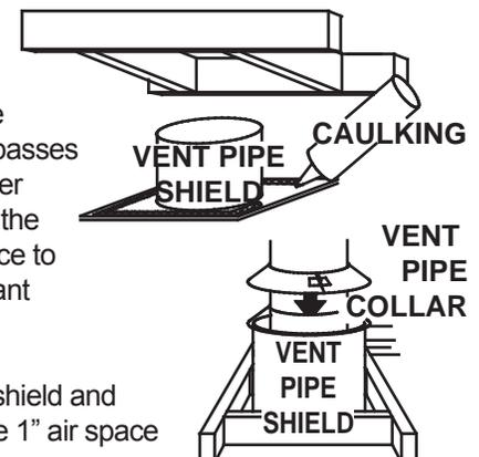
C. In the attic, slide the vent pipe collar down to cover up the open end of the shield and tighten. This will prevent any materials, such as insulation, from filling up the 1" air space around the pipe.
