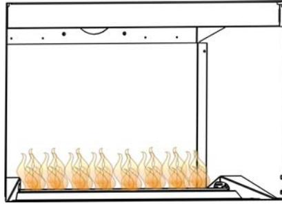
**FLAME MUST ENVELOP UPPER 3/8" TO 1/2" OF FLAME SENSOR**
