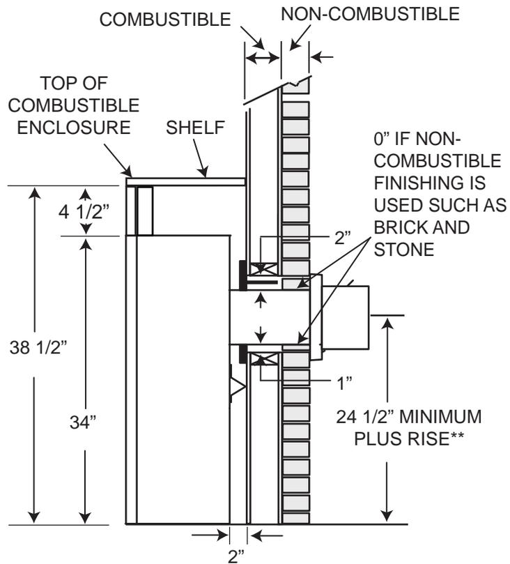
The appliance requires a minimum enclosure height of 38 1/2" (REAR VENT) 49" (TOP VENT). For temperature requirements, the enclosure space around and above the appliance must be left unobstructed.
