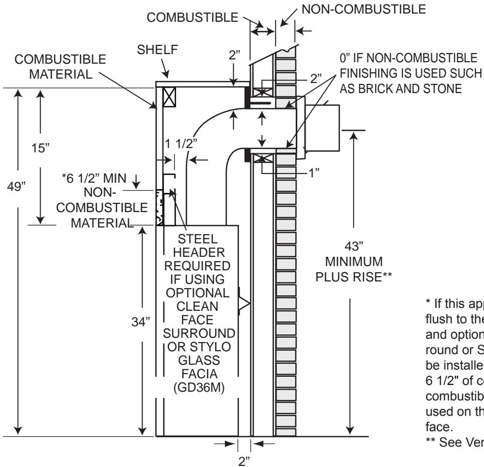
\* If this appliance is installed flush to the finishing material and optional clean face surround or Stylo glass facia is to be installed then a minimum of 6 1/2" of cement board or non-combustible equivalent must be used on the top only of the front face.
