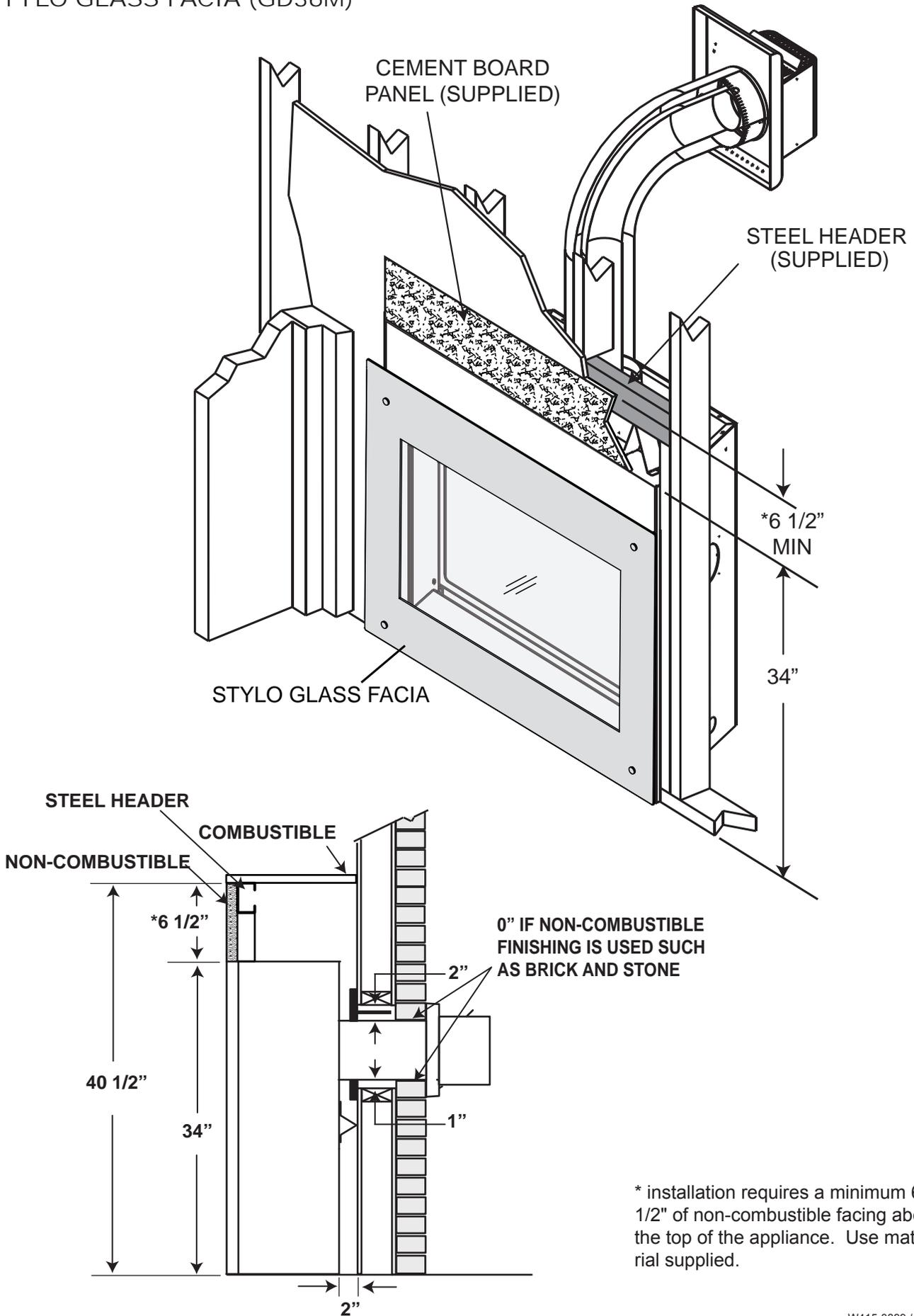
\* installation requires a minimum 6 1/2" of non-combustible facing above the top of the appliance. Use material supplied.
