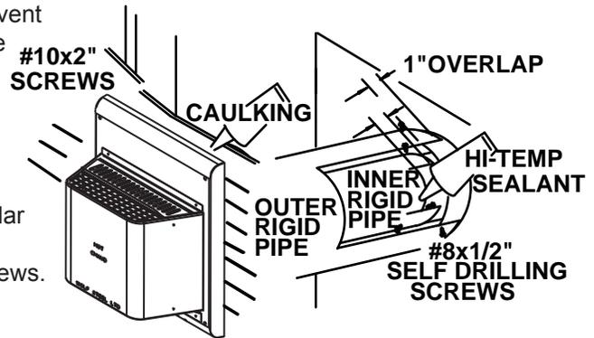
**The air terminal mounting plate may be recessed into the exterior wall or siding no greater than the depth of the return flange.**
