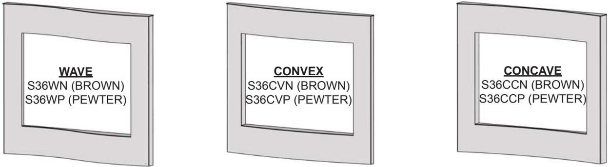
Installation requires a minimum of 6 1/2" non-combustible facing material at the top of the appliance. Refer to illustrations above (depending on your installation) to ensure your appliance has been installed with the proper requirements for this kit.
