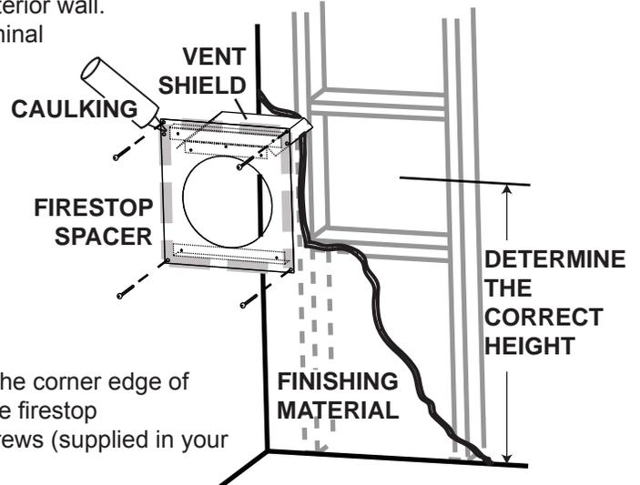
A. Apply a bead of caulking (not supplied) around the corner edge of the inside surface of the firestop assembly, fit the firestop assembly to the hole and secure using the 4 screws (supplied in your manual baggie).
