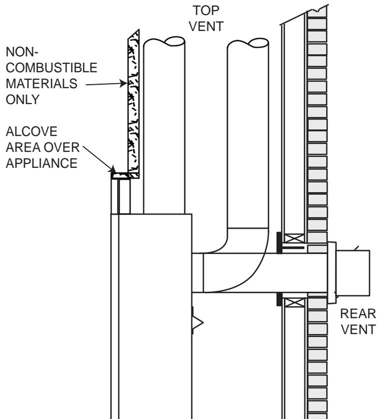
Alcoves above the appliance can be made as deep as desired as long as the clearances to combustibles are maintained as in 6.3.1 and 6.3.2. If clearances to vent components are reduced, materials must be non-combustible.
