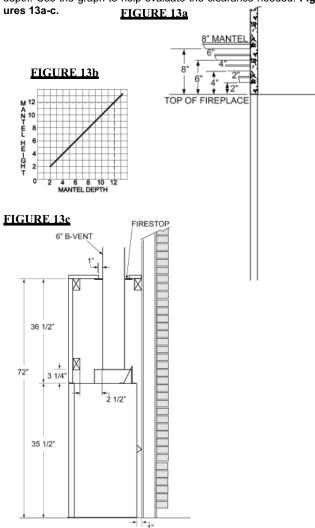
The fireplace requires a minimum enclosure height of 72". For temperature requirements, the enclosure space around and above the fireplace must be left unobstructed.
