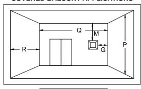
$Q_{MIN}$  = 3 feet  $R_{MAX}$  = 2 x  $Q_{ACTUAL}$  $R_{MAX}$  ≤ 15 feet
