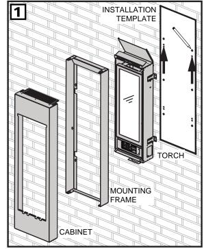
**B.** Remove the template. Depending on the surface and fasteners, drill the appropriate holes. Hold the Torch up, aligning the mounting brackets to the mounting holes. Secure the Torch to the wall using the appropriate fasteners.
