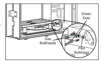
B. Connect the pilot electrode leads to the bulkhead. The leads can only fit one way. You need to match the 1/4" flag with the 1/4" bulkhead spade and the 3/16" flag with the 3/16" spade.
