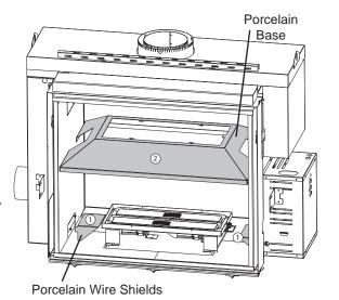
C. Align the 4 tabs on the porcelain base 2 down to line up with the holes in the burner tray. Secure using the screws provided.
