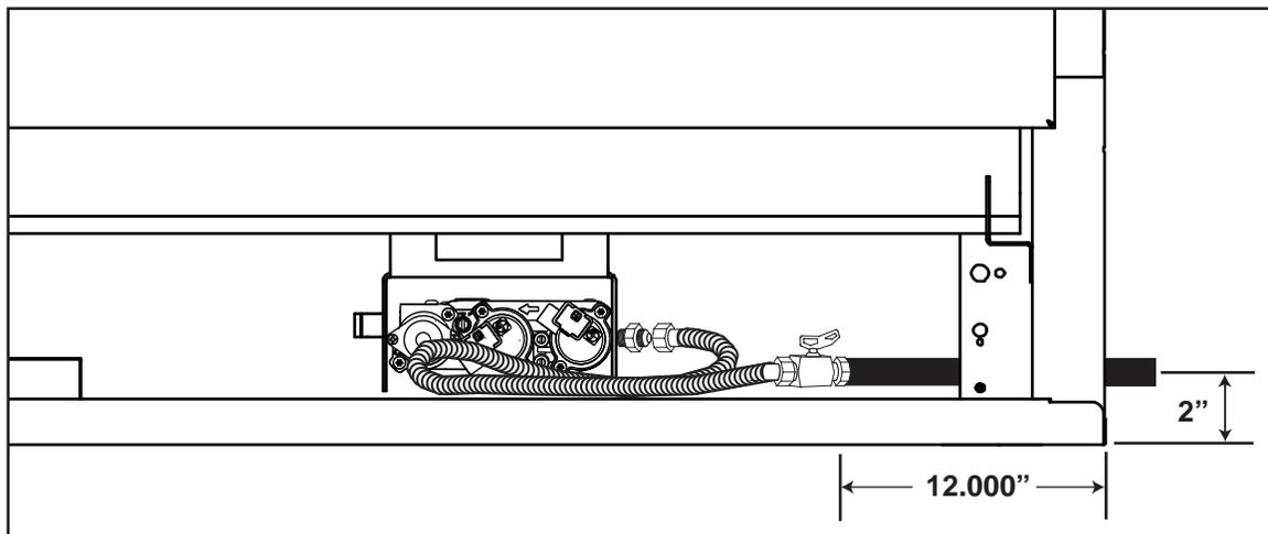
**NOTE:** Connect the gas supply to the 1/2" shut off and flex connector (supplied). Ensure gas supply is secured and that there is sufficient movement of the connector to permit lifting the burner base assembly for component servicing.
