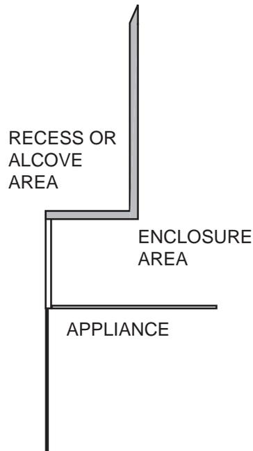
**NOTE:** Recesses or alcoves above the appliance can be made as deep as desired provided the minimum clearances to combustibles are maintained.
