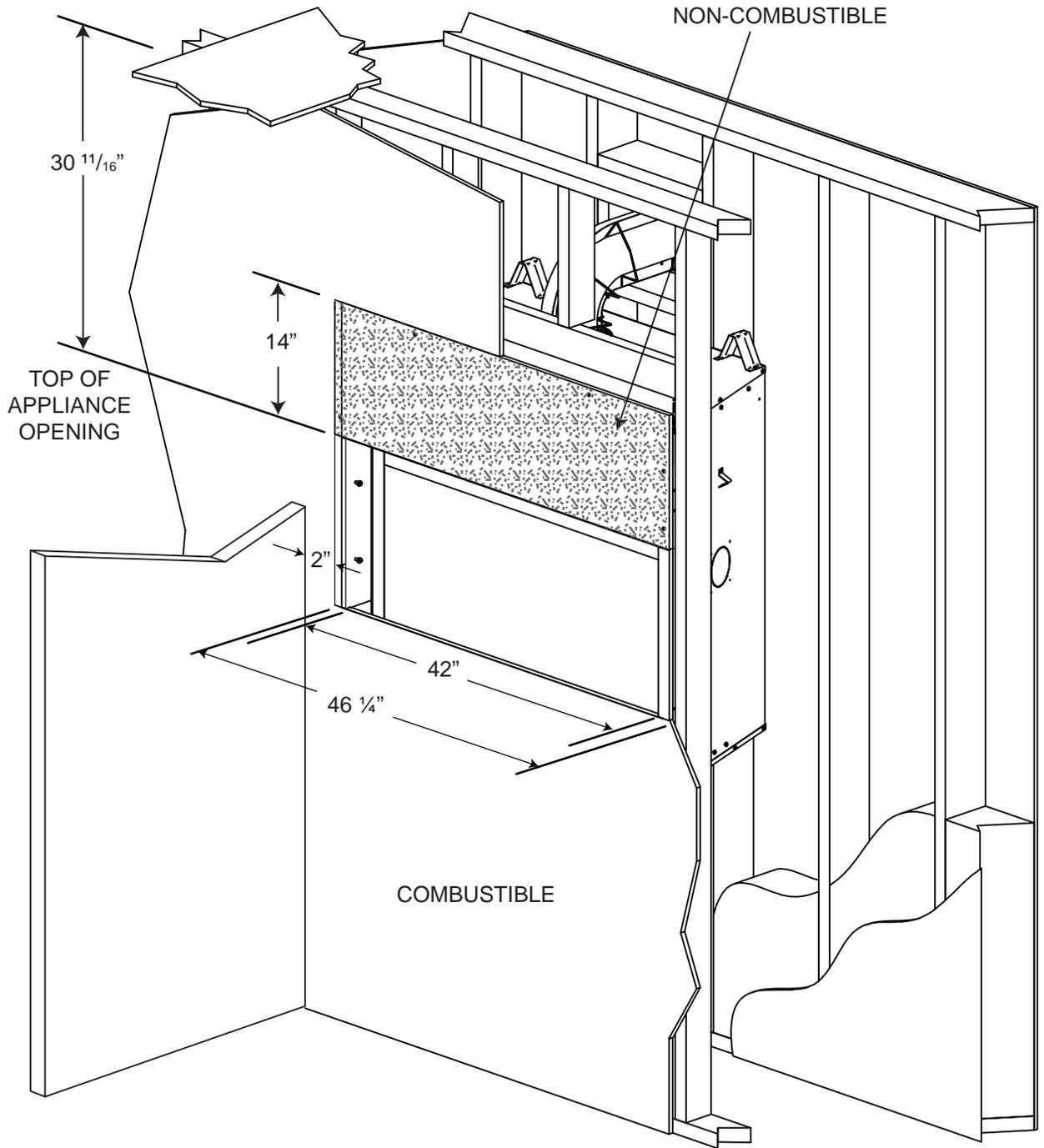
Finishing material may be secured directly to the appliance body where practical.
