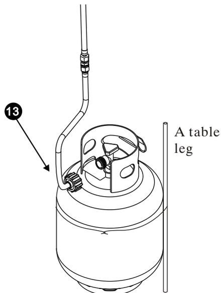
**WARNING : TO BE INSTALLED ONLY BY AN AUTHORISED PERSON****Step 7 ---- Check for leak**
