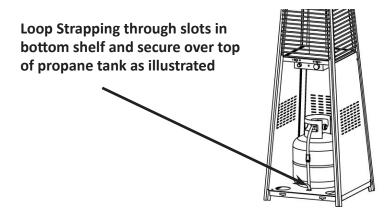
Cylinder Connection: Ensure the gas regulator hose is kink free. Remove the cap from the cylinder fuel valve. Insert the black QCC1 regulator nipple onto the QCC1 fuel valve. Hand tighten clockwise. Do not use tools. Leak test all joints prior to using the patio heater. A leak test must be performed annually and each time a cylinder is hooked up or if a part of the gas system is replaced.
