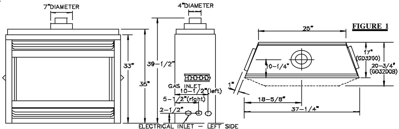
*Provide adequate ventilation and combustion air. Provide adequate accessibility clearance for servicing and operating the fireplace. Never obstruct the front opening of the fireplace.*
