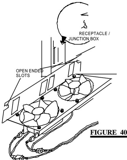
The wire harness provided in this kit is a universal harness. When installed, ensure that any excess wire is contained, preventing it from making contact with moving or hot objects.
