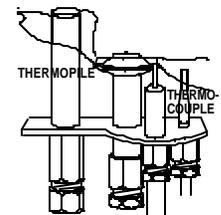
FLAME MUST ENVELOPE UPPER 3/8" TO 1/2" OF THERMOCOUPLE & THERMOPILE
