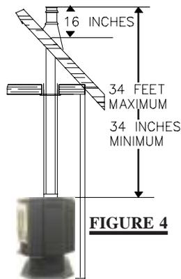
**Use an adjustable pipe as the final length of rigid piping to the stove for ease of installation.**
