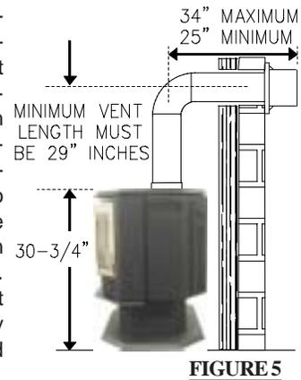
The maximum horizontal run is 34 inches with a 90° elbow located 29" above the stove. **FIGURE 5.**
