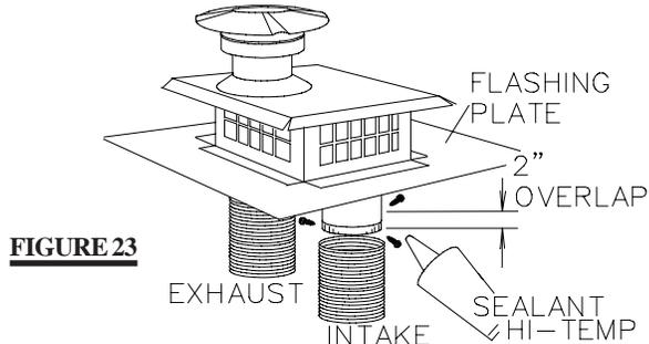
Chimney installation must conform to both national and local code requirements. The chimney must be lined with two 3" diameter liners. The minimum and maximum liner lengths are 10 and 35 feet respectively. Recommended Napoleon kits come in 3 lengths: 20 foot (GDI-320KT), 25 foot (GDI-325KT), and 35 foot (GDI-335KT). While the liners must be continuous from the fireplace to the chimney cap, to achieve the needed length, they may be coupled, using an approved coupler.
