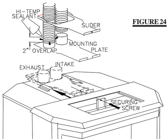
3. **INSIDE:** Remove the securing screw from the front of the vent mounting plate. (The screw can be accessed through the trivet opening.) Remove the vent mounting plate and the slider from its track. **FIGURE 24.**
