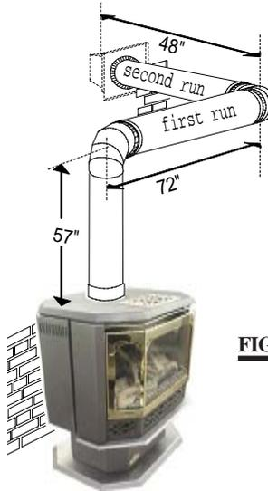
If a first run of 72 inches is required, using the "First Vent Run" on the chart shows that a maximum second run of 48 inches is allowable.
