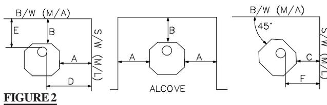
No additional floor protection is required minimum 20" from stove top to ceiling
