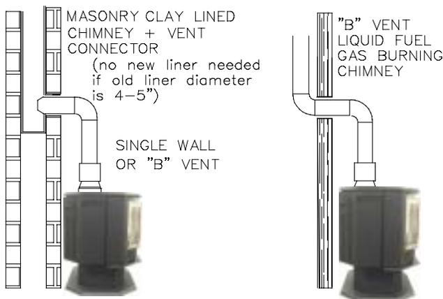
A CHIMNEY VENTING THIS STOVE SHALL NOT VENT ANY SOLID FUEL BURNING APPLIANCE.
