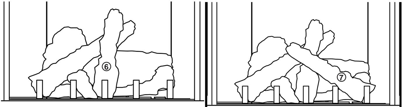
Position the notch located in log #6 against the grate post.
