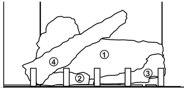
Place log #1 onto the burner, centering it onto the burner tray and pushing it as close to the rear wall of the firebox as possible. Move logs # 2 and 3 into position, lining up the studs located on the burner with the holes on the bottom of the logs. Sit the notch at the bottom of log #4 against the left outermost grate post and position the top of the log into the pocket provided on the rear log (#1).
