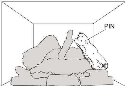
**10.** Position the right crossover log over the pins in the right side of the middle and rear logs. Place a pin in the top of the log.
