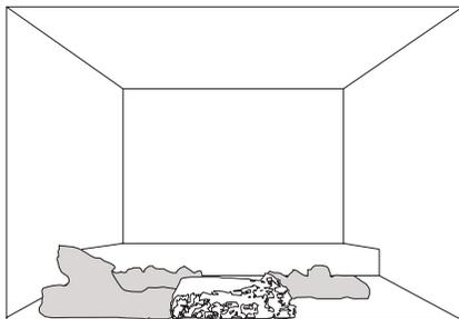
**4.** Place the centre charcoal piece\* into position, lining up the hole in the bottom with the stud in the front centre of the log support.
