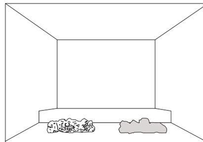
**2.** Place the left charcoal piece into position, lining up the bottom holes with the studs to the left side of the burner.
