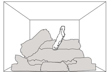
**9.** Position the middle crossover log onto the middle pin of the rear log. Rest the end of the log into the notch of the middle log.
