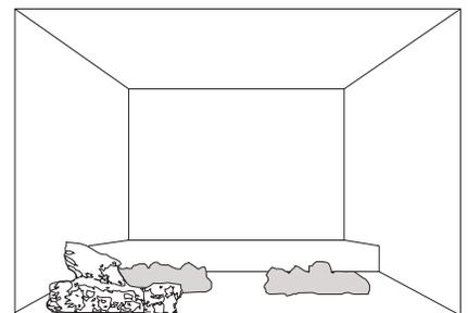
**3.** Place the left front charcoal piece\* into position, lining up the holes in the bottom with the studs in the left front corner.
