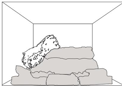
**8.** Position the left crossover log over the pins in the left side of the middle and rear logs.
