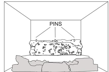
**6.** Place the rear log against the back panel, lining up the holes with the studs at the back of the firebox. Locate 3 pins (supplied) into the top of the log.
