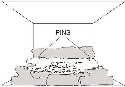
**7.** Position the middle log behind the burner pan, lining up the holes with the 4 studs, ensuring the log is flat against the base. Place 2 pins into the left and right top holes.
