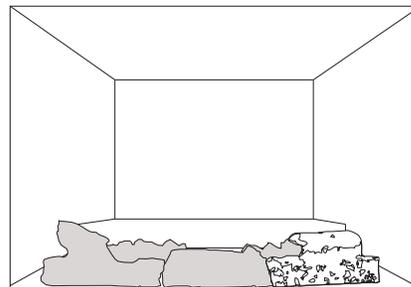
**5.** Place the right front charcoal piece\* into position, lining up the holes in the bottom with the studs in the front right corner.
