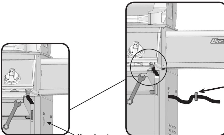
Ensure bushing snaps into side panel as shown.
