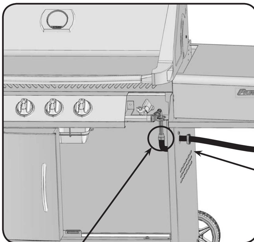
Ensure bushing snaps into side panel as shown.
