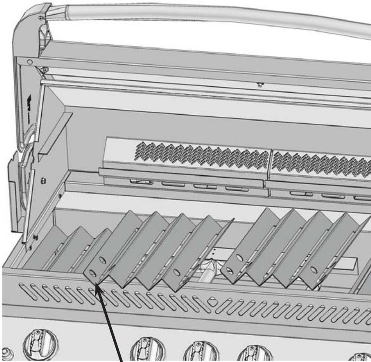
Ensure holes in sear plates are positioned to the front of the grill.
