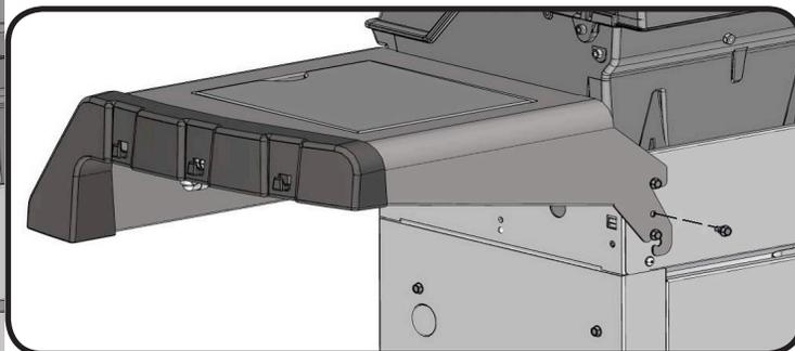
**Side Burners must be locked in place
