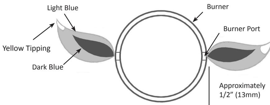
**Burner:** The burner is made from heavy wall 304 stainless steel, but extreme heat and a corrosive environment can cause surface corrosion to occur. This can be removed with a brass wire brush.
