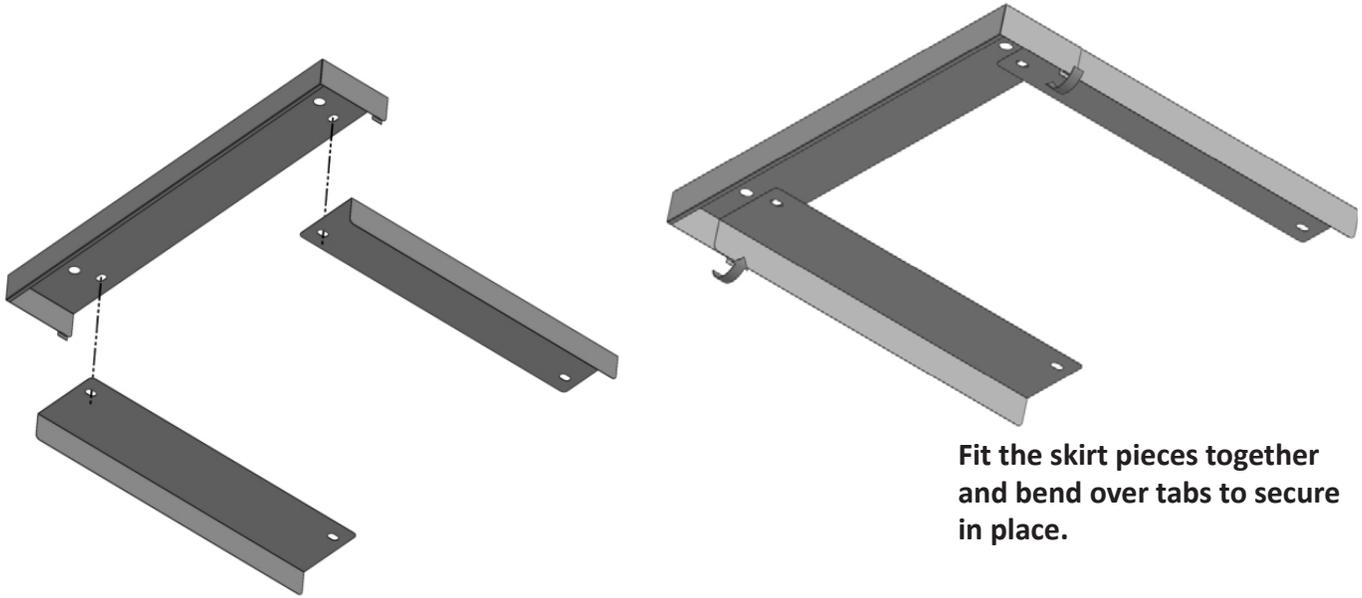
Fit the skirt pieces together and bend over tabs to secure in place.
