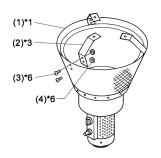
Before assembling the burner head on post, please fix the 3 supported brackets onto burner head for assembling reflector
