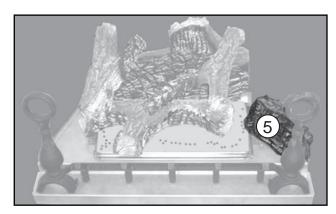
E. Position the slot in the bottom of log #5 onto the bracket beside the burner on the right, and against the back side of the andiron with the charred face of the log to the front.
