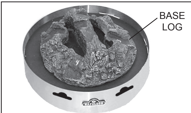
4.1.1 Set base log onto burner ensuring stud and bracket fit into hole and notch. Base log should sit flat on "Patioflame" base.
