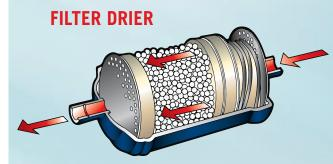
Napoleon air conditioners are built to include the highest quality filter drier in the industry. A filter drier is an extremely beneficial component to your system. Working to remove unwanted acids, dirt, particle debris and other contaminants from the refrigerant, the filter drier extends the life of your air conditioning system.
