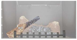
6.2.3 Place the bottom of the left crossover log (#4) against the left firebox side and pulled forward to the grate. The top of the log should rest in the pocket on the back log.
