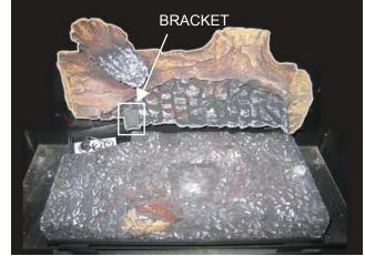
A. Place the rear log, as shown, onto the rear log support brackets. Ensure the cutout on the left underside of the log, fits over the pilot-assembly. Bend the bracket on the left side to help retain the rear log.
