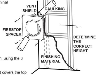
A. Assemble the shield to the spacer as shown, using the 3 shorter screws supplied.
