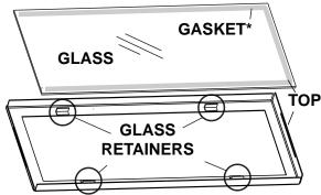
\* When installing the door glass ensure that the gasketed end is placed into the top of the door frame.
