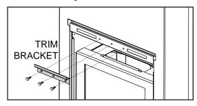
5.4.2 Install the trim bracket supplied in your manual baggie to the firebox using 3 screws.
