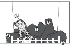
Line up the rectangular hole in the left crossover with the rectangular post located on the left side of log and install as shown.
