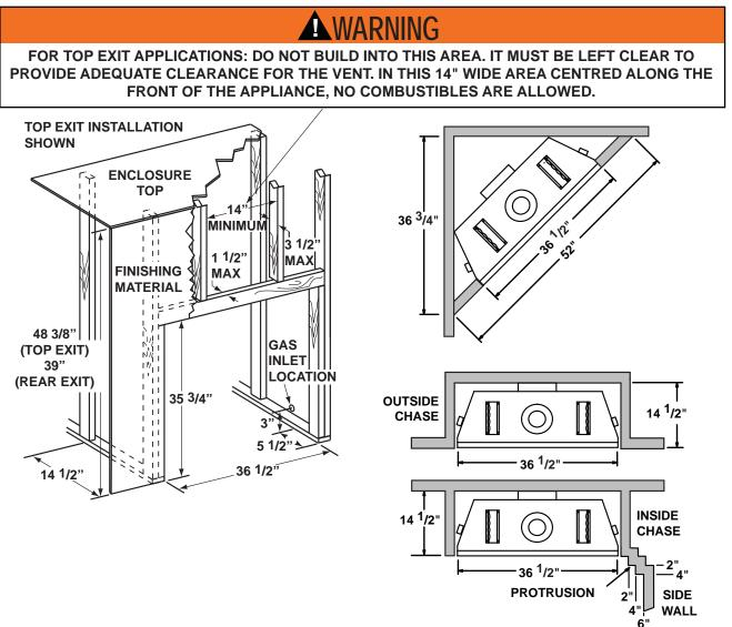
Combustion protrusions such as mantels and shelves may occur at or after a minimum distance of 2" away from the side of the appliance. Thereafter, the depth of any protrusions must be equal to or less than the distance from the side of the appliance up to a depth of 6", after which no greater clearance than 6" is required. This can be considered a side wall with no length boundary.
