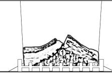
A. Place the rear log so that it rests against the two log brackets on the back wall of the firebox. The air space between the log and firebox back is used to facilitate combustion air flow.
