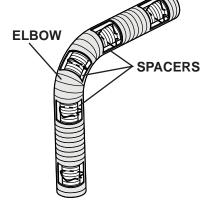
All inner flex pipe and outer flex pipe joints may be sealed using high temperature sealant W573-0002 (not supplied) or the high temperature sealant W573-0007 Mill Pac (not supplied). However, the high temperature sealant W573-0007 Mill Pac (not supplied) must be used on the joint connecting the inner flex pipe and the exhaust flue collar. **Use only approved flexible vent pipe kits marked:**
