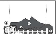
**D.** Move the left log into position lining up the hole in the bottom with the stud on the left side of the log support.
