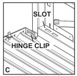
LOWER LOUVRES Insert the hinge clips into the slots located at the bottom left and right corners of the unit. To remove the louvres, pull the back tabs of the clips forward, while pushing the louvre assembly back. Lift the clip. 57.2
