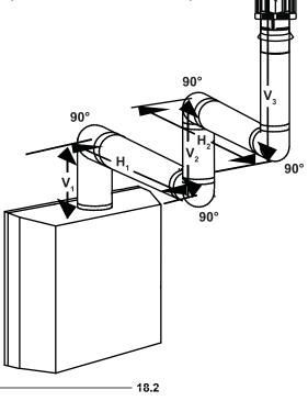
$(H_{T}) > (V_{T})$ See graph to determine the required vertical rise  $V_{\tau}$  for the Simple venting configurations. required horizontal run H<sub>-</sub>. 19 REQUIRED VERTICAL **RISE IN** FEET V<sub>T</sub> 0 5 10 15 20 25 30 HORIZONTAL VENT RUN PLUS OFFSET IN FEET H<sub>T</sub> The shaded area within the lines represents acceptable values for H<sub>+</sub> and H<sub>+</sub>
