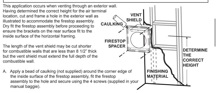
B. Once the vent pipe is installed in its final position, apply high temperature sealant W573-0007 (not supplied) between the pipe and the firestop.
