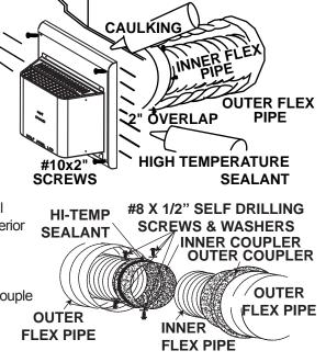
The air terminal mounting plate may be recessed into the exterior wall or siding no greater than the depth of its return flange.
