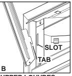
**UPPER LOUVRES** Insert the louvre tabs into the slots located at the top left and right corners of the unit.
