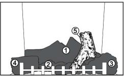
E. Line up the square hole in the right crossover with the square post located on the right side of log and install as shown.
