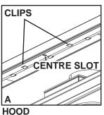
Attach the hood by pressing the top flange into the clips along the top of the louvre opening. Secure using a screw through the centre slot.
